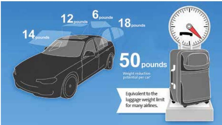
**Figure 2.** Using glass glazing that is ~30% lighter can reduce vehicle weight by as much as 50 pounds, as calculated by Corning for a sport utility vehicle featuring Gorilla Glass hybrid laminate windows.
